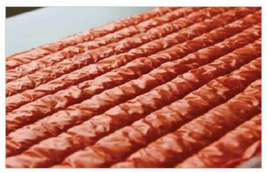
A new synthetic alternative to down, Thermore ARIA ("air" in English) is 98 percent air by volume, ultra-light, soft and a super efficient high-loft insulator. Image: Thermore.
